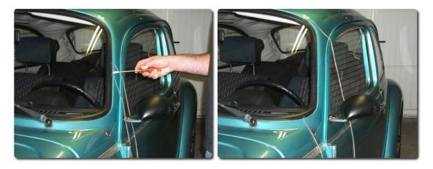
Now, take the A-pillar deflector and remove a small piece of the protection of the double sided tape. Fold this piece in a corner so that it just comes out under the deflector.
