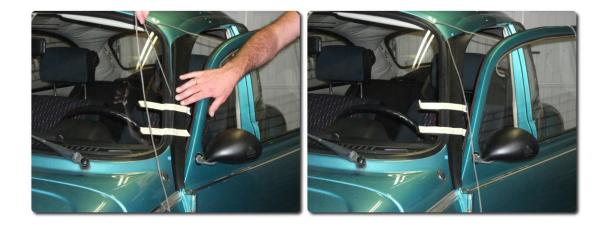
When the deflector edge is under the rubber, ensure that it is under the rubber far enough. Now you can position it in the right location.
