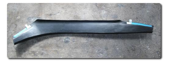
This allows you to position the deflector before you remove the protection of the tape and it sticks to the car.
